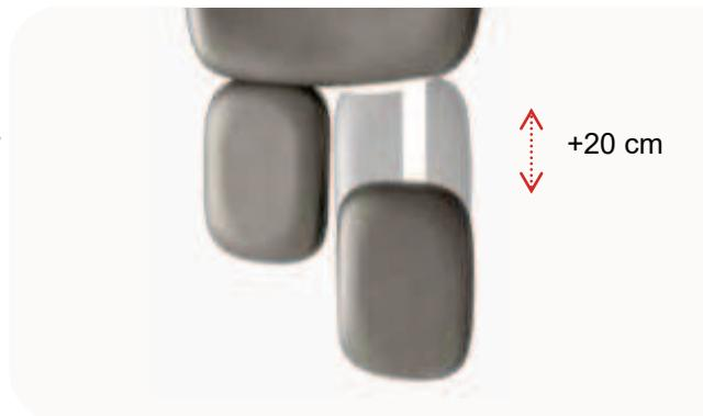
The leg-rest can stretch 200mm on its support axis.
